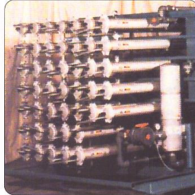
Reverse osmosis grooved end caps allow easy filter membrane service
